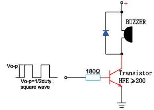
The base current Ib should high enough so that it saturates the collector current of the transistor with the CB load.
